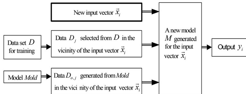
Fig.2 A block diagram of a transductive inference system. An individual model  $M_i$  is trained for a new input vector  $\bar{x}_i$  with data samples  $D_i$  selected from a data set  $D$ , and data samples  $D_{o,i}$  generated from an existing model.
