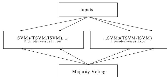
Fig. 3 The structure of SVM ensemble for promoter recognition
