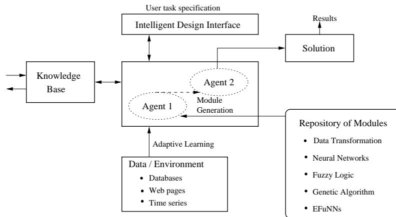
**Fig. 2.** A block diagram of an agent-based, adaptive intelligent decision support system – HIDSS that uses the architecture of an AIES.
