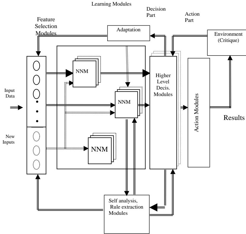
**Fig. 3.** A block diagram of the general framework of the EMU-HIDSS as an evolving connectionist-based system (adapted from [22]).
