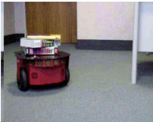
Figure.1 ROKEL is built with the use of Pioneer 2 DX robot hardware platform
