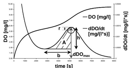
Figure 5. Characterisation of a breakpoint in the DO profile through five geometrical features: Area (A), height (h), maximum value ( $dDO_{max}$ ), width (b), curvature radius at the top (r).
