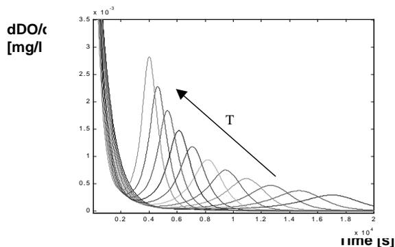
Figure 4. Effect of temperature on the shape of the peak in the first derivative of the dissolved oxygen at the end of nitrification (mathematical model).
