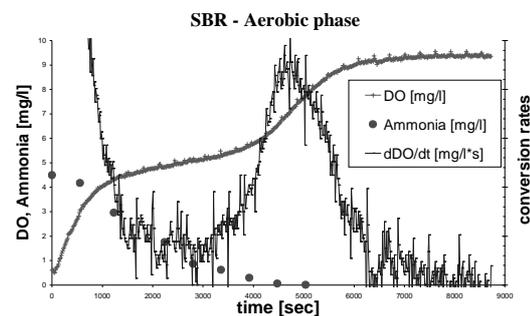
Figure 3. Dissolved Oxygen and ammonia concentration measured in a SBR during the aerobic phase
