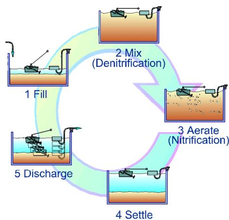
Figure 1. Sequencing Batch Reactor (SBR) Process
