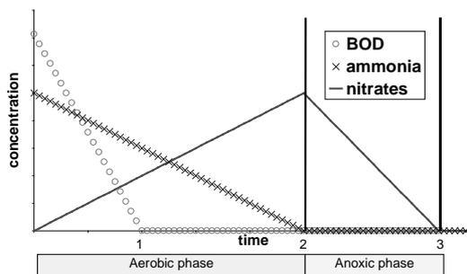
Figure 2. Removal of polluting matter in a SBR.
