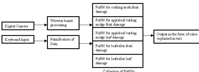
Figure 9: Overall architecture of the HortResearch Pest Identification System
