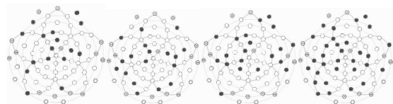
Fig.4. The location of the selected electrodes for each of the stimuli of classes from 1 to 4 (from left to right respectively)
